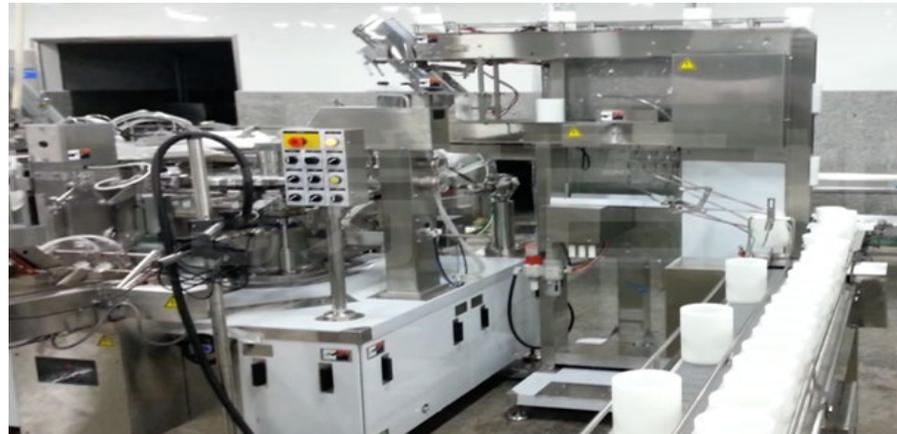
Ingredients filling equipment (small pouches for B2C)
